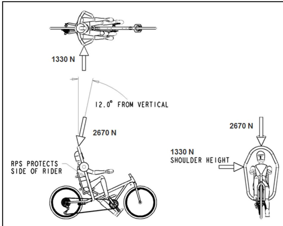
**Figure 1: Example of Proper RPS Design and Side and Top Load Case Applications (Note: Loads shown should not be applied concurrently in analysis and/or testing. Reaction loads should be applied at safety harness attachment points)**
